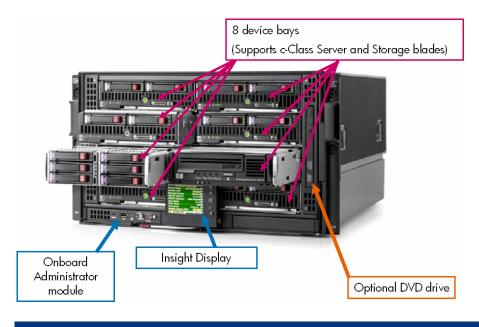
Figure 2. HP BladeSystem c3000 Enclosure - rear view
